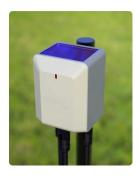
The TRU is a maintenance free, solar powered, field unit. 2 valve RTU operates up to 2 independent valves, 4 valve RTU operates up to 4 independent valves, designed for outdoor use with multiple mounting options. The RTU can also sample and relay the reading of one sensor, analog soil moisture sensor or any switch type sensor.
