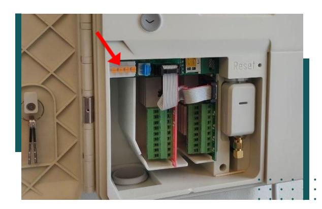
The terminal to the left corresponds to Base Sensor 1, the other terminal is sensor 2.
