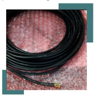
The cable should not be modified by the customer. It is not possible to shorten or extend an RF cable without severely undermining radio performance. If your requirements can not be met with the 10m cable between the antenna and the Base Unit, please order a cable with desired length from us or other electronics/radio professionals. The cable has an N-type socket on the antenna side and SMA plug on the Base Unit side. The Base Unit has two RF ports, both residing on top of the unit.
