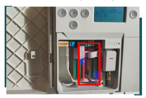
Pull the wires through the inlet cover underneath the unit. Pull out the Extension board to access the terminal's screws. Screw the wires (no polarity). Push the board back in, when the wires are connected.
