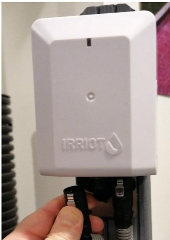
Carefully disconnect the valve and, if applicable, also the sensor connection cables from the unit. Push the metal latch on the contact with your thumb while carefully pulling it out from the body. *Please see the picture.*
