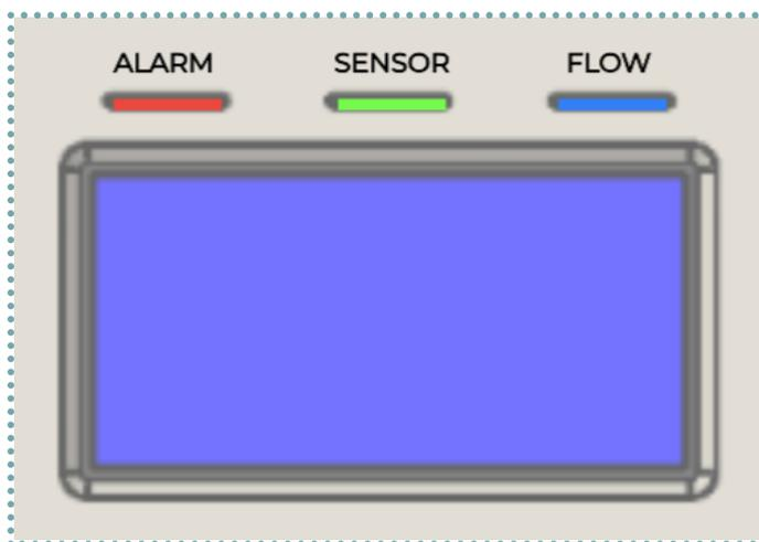
The Base Unit has three LEDs on the front panel. Upon power up, all three LEDs are illuminated for approx. 2 seconds.
