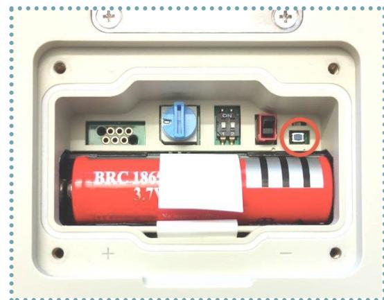
**Important:** pay attention to the pairing LED on the RTU when you push the pairing button. If, when you push the pairing button, the LED is steady on for a couple of seconds, then is off, this means you have succeeded. The pairing is now completed.
