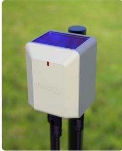
The **Remote Terminal Unit (RTU)** is maintenance free, solar powered, field unit, 2 valve Remote Unit operates up to 2 independent valves, 4 valve Remote Unit operates up to 4 independent valves, designed for outdoor use with multiple mounting options. The Remote Unit can also sample and relay the reading of one sensor, analog soil moisture sensor or any switch type sensor.
