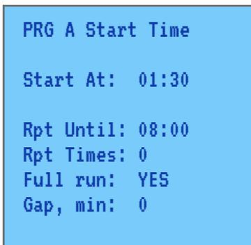
**Start Time** is when the program starts executing the watering sequence. The program can repeat the sequence a number of times per day if you define multiple **Start Times** or configure repetition options: **Repeat Until** or **Repeat Times**. If no **Start Time** is defined, the program can only be **executed manually**.
