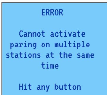
**Only one wireless station (RTU)** can be set for pairing at a time. If you try to set another wireless station in pairing an **ERROR** message will be displayed.
