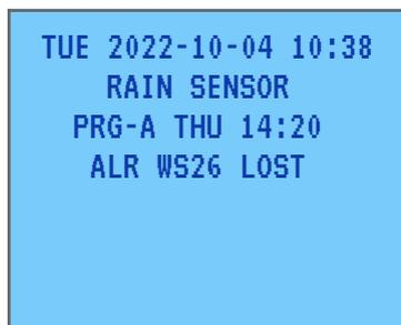
In Idle state the **Main Screen** displays the current status of the IRRIOT system, as well as the scheduled irrigation occasions. The idle state is the default state upon power-up.
