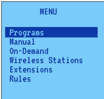
The menu has multiple levels. Use the arrow buttons on the left hand side to scroll up and down the items. To enter an item press the **OK** button. To come one level up press the **Back** button. When the **Back** button is pressed in the main menu (highest level) the Menu state is quit and the LCD returns to the Idle state.
