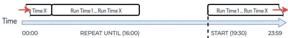
The parameter **Gap**, if defined, is the time in minutes to be idle between subsequent repetitions within the time window between **Start Time** and **Repeat Until** time. Please see the picture below.
